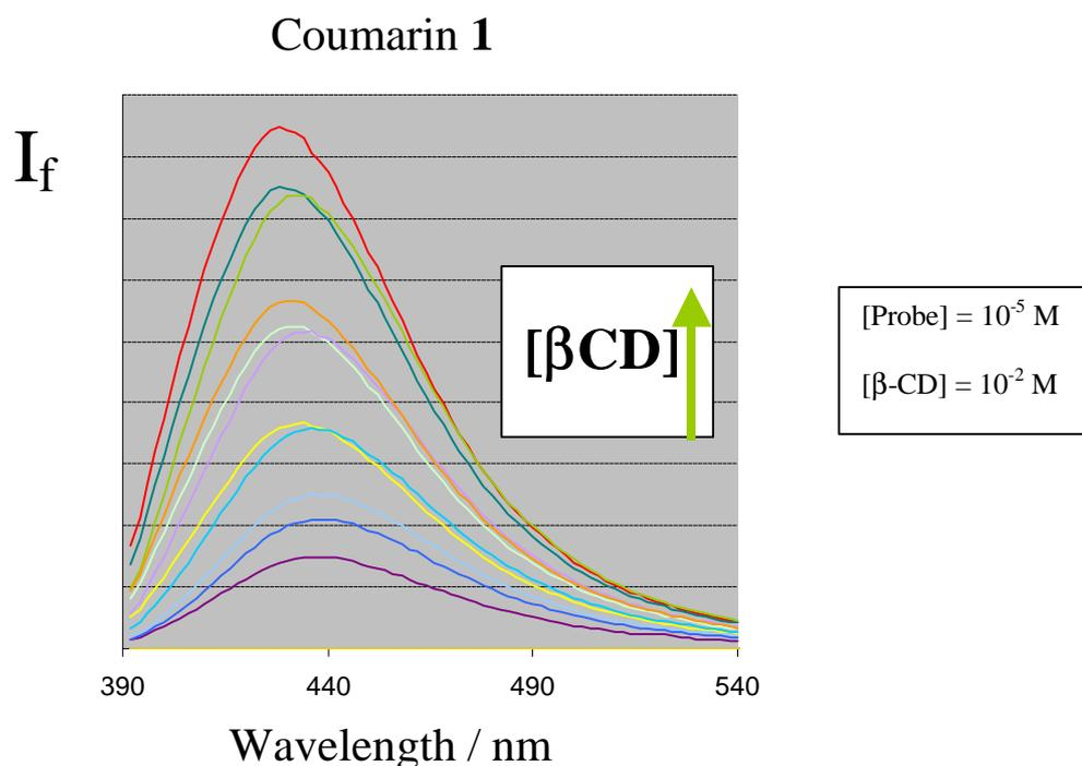
A **blue-shift** was also observed in the presence of  $\beta$ -CD, together with an **increase of the lifetime**. This indicates that the dye was localized in a medium less polar than water, and that its excited state was stabilized.
