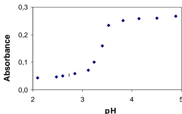
Addition of  $\beta$ -CD in aqueous solutions of **1** and **2** induced a weak **hypochromic shift**. No effect was observed with  $\alpha$ -CD and  $\gamma$ -CD.
